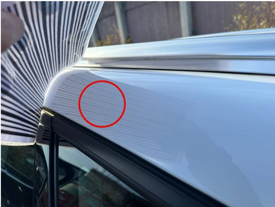
Kleine Delle Dachholm links
